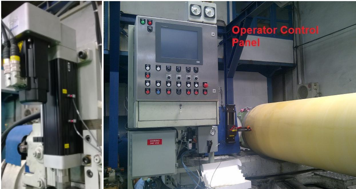
Pictures: RollTrack® servo control system installed on the Farrel two-wheel roll grinder.
