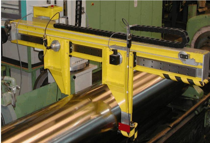
A machine mounted model is custom designed for a roll grinder.
