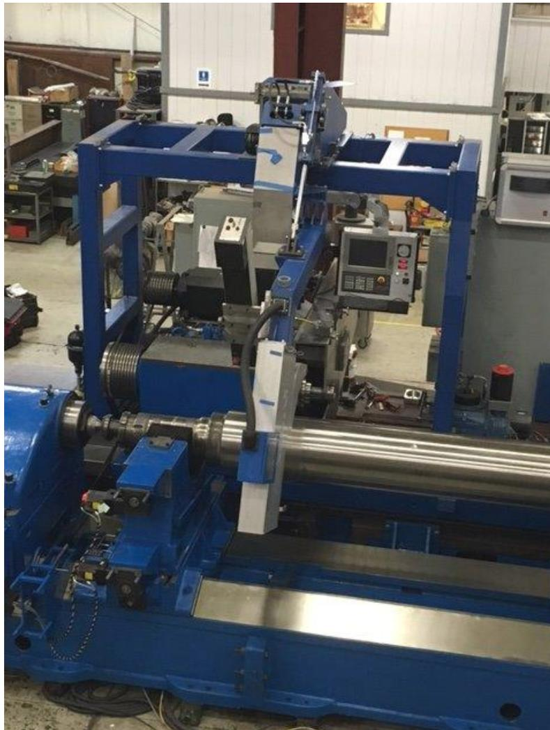
Pictures: In process gauging: roll measurements are taken when grinding and FMT RollTrack® sends the results to the CNC control for error compensation. The caliper hardware was designed and manufactured by WMG. Eddy current fault detection system is mounted on the same arm assembly. Abbott Machine rebuilt the above roll grinder.
