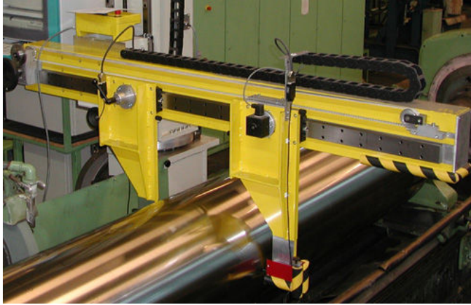
Figure 1. PWT machine mounted roll caliper with two measuring probes.
