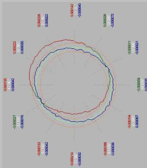
A measurement graph on a new roundness measurement procedure from a single gauge T.I.R. measurement. The graph shows that the roundness measurement result is within +/- .0001" (2.5µm) tolerances after eliminating run-out from a T.I.R. measurement at the roll center.
